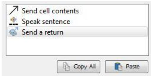
You can copy the assigned Actions from any Cell or Button for the purpose of adding them to others. This is particularly useful when you have many Cells in an Environment that you wish to function in the same way.
